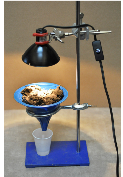
Complete setup with ring stand, light and funnel.
