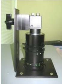
**Figure E-6:** *Adjusting the Focus Ring*
