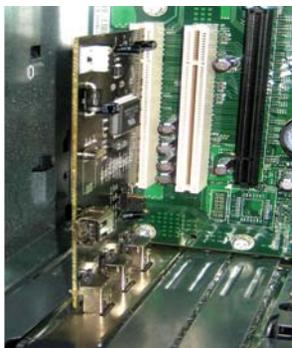
*Figure D-6: Connecting Firewire Cable to the Firewire Card*
