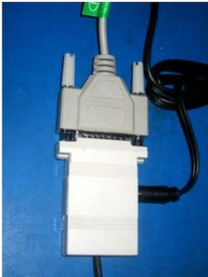
**Figure D-5:** Connecting the Motorized Lens Power Supply
