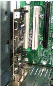
**Figure E-7:** *Connecting Firewire Cable to the Firewire Card*
