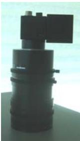
**Figure E-5: Attaching Spacer Block to Camera**
