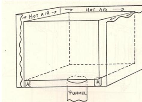
FIGURE 2. DRYING STOVE WITH THE FRONT WALL AND LID REMOVED SHOWING INTERIOR OVEN SUPPORTED BY BLOCKS (A).
