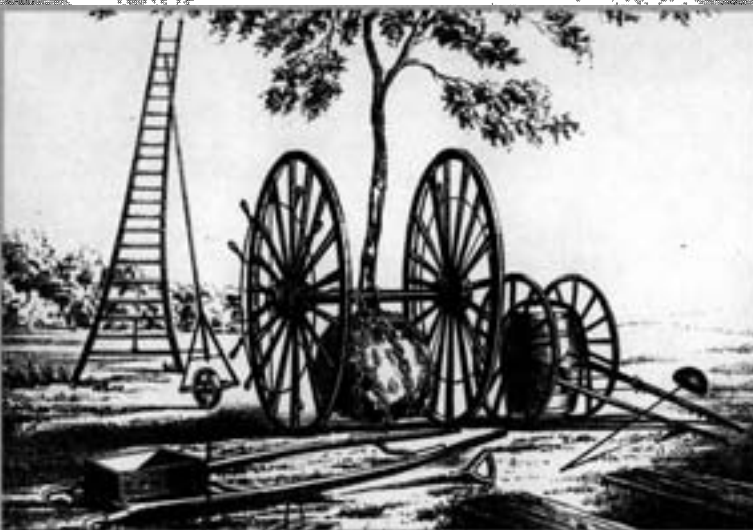
Tree moving equipment circa 1853. Illustration from The Tree Lifter, by Colonel George Greenwood.
